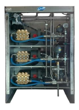
This hydraulic high pressure washer includes three high pressure water pumps which delivers 40l/min each at 170 bar. Piping and cabinet is made of stainless steel. See-through splash guard in front.
